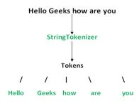
A StringTokenizer object internally maintains a current position within the string to be tokenized. Some operations advance this current position past the characters processed. A token is returned by taking a substring of the string that was used to create the StringTokenizer object.
