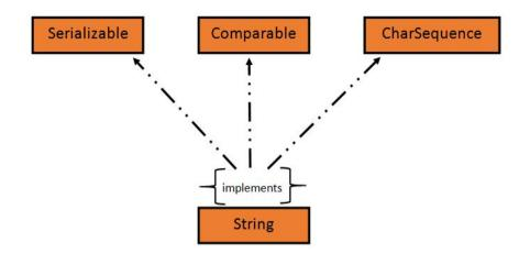
In Java, **CharSequence** Interface is used for representing a sequence of characters. CharSequence interface is implemented by String, StringBuffer and StringBuilder classes. This three classes can be used for creating strings in java.
