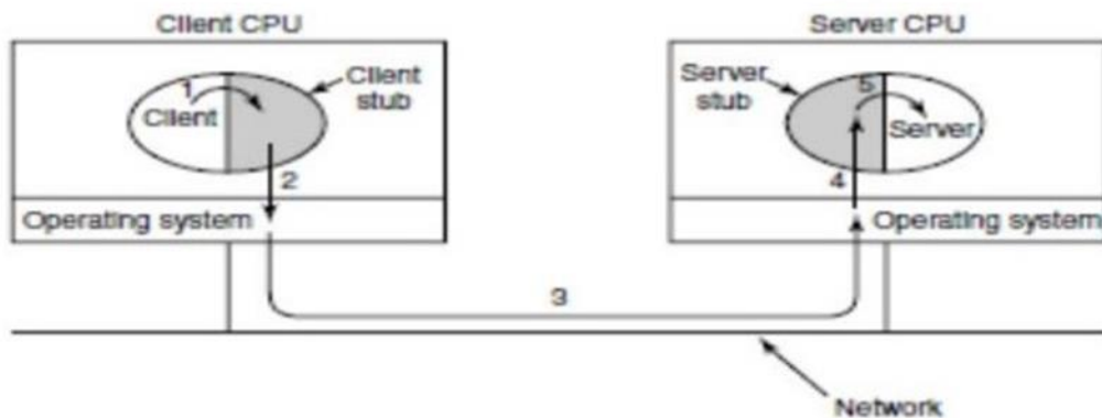
Steps in making a RPC
